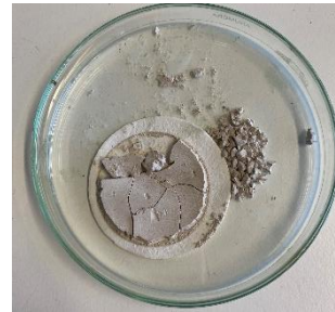
Precipitate from process water from HTC at 250 °C
